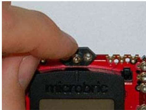
**Step 2** > Place the sounder module onto the bric.
