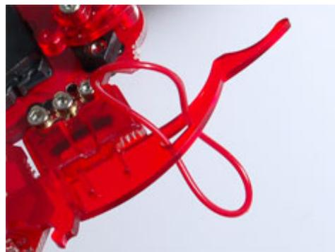
**Step 10>** Push the bottom half of the rubber band up through the top half.
